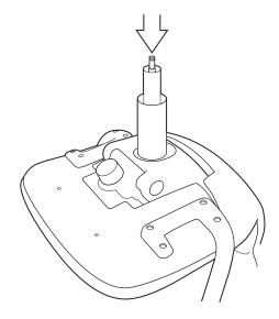
4) Place washer, bearing, second washer and rubber washer over end of gas cylinder strut.
