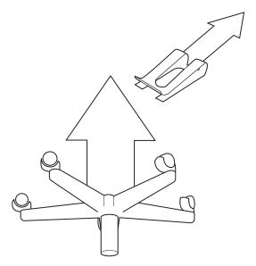
2) Using a small flathead screwdriver remove the ring locking cylinder in support tube and pull gas cylinder out of tube.
