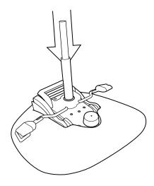
6) Place washer, bearing, second washer and rubber washer over end of gas cylinder strut.
