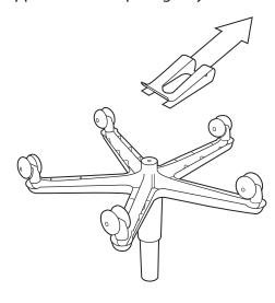
2) Using a small flathead screwdriver remove the ring locking cylinder in support tube and pull gas cylinder out of tube. Note: You will not be able to re-use this ring but a new lock-ring is provided with your new gas cylinder kit.
