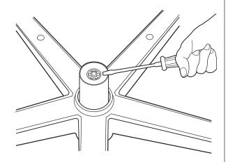
If the original star base is a press fit design use a rubber mallet or soft tool to loosen it from the cylinder.
