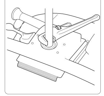
4) Star bases may be press fit or require a lockclip. If a lock-clip is required, the black outer cover of the gas cylinder may be removed.
