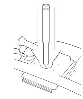
2) With the star base removed twist base of the cylinder using a pipe wrench. It may require significant effort to break the old cylinder free.
