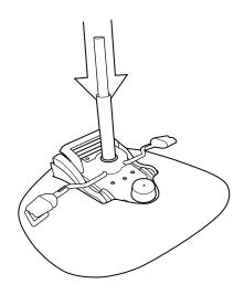
6) Place washer, bearing, and second washer over end of gas cylinder strut.
