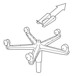
2) Using a small flathead screwdriver remove the ring locking cylinder in support tube and pull gas cylinder out of tube. Note: You will not be able to re-use this ring but a new lock-ring is provided with your new gas cylinder kit.
